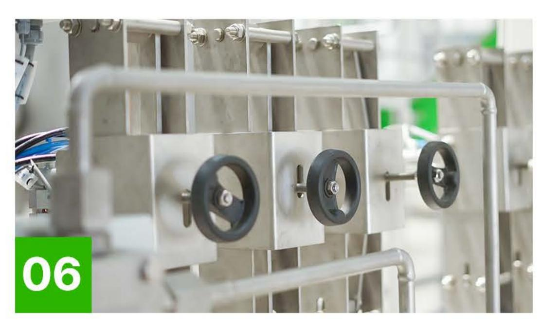
Proprietary Changeover Valves for quick changeovers and isolations, even at high pressures
